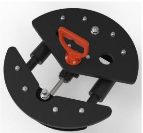
The GNT Solutions AS **Hydraulic AX-VX Gasket Tool** is designed to give the operator an effective and simple method of removing/installing an AX- or VX-Gasket by using a ROV. A spring-loaded failsafe assembly, together with the lower locking plate in the sandwich assembly ensures that the AX- or VX-Gasket cannot be lost/dropped out of the tool by accident. The tool must be hydraulically operated to unlock and release the gasket.
