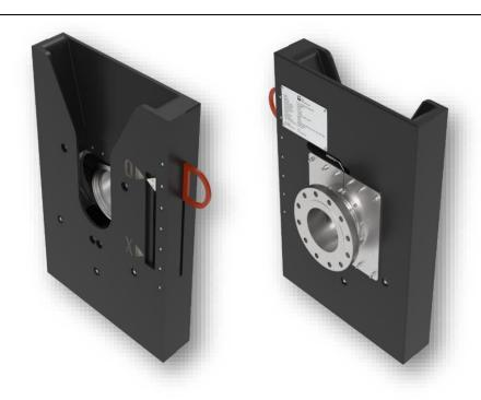
The **Subsea Pressure Connectors** are ROV operated connectors intended for temporary or permanent installations subsea. They have dual seals and a seal test -port. All flange interfaces and materials can be adjusted to fit customer needs.
