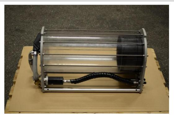
The **Acid Injection Cylinder** can be used with a 18-3/4" AX/VX Cleaning Tool system. The acid is supplied by an ROV driven pump into the connection point on the tool.
