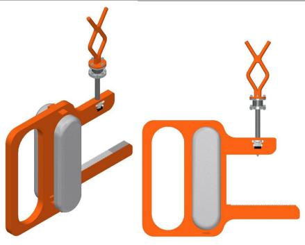
The **Subsea anode clamp** is a universal anode clamp that can be mounted on metal surfaces. The clamp opening is placed onto the structure and secured in place by operating the ROV handle. The structure is designed tension up when the handle is turned and tightened up. This in combination with two-disc springs in the ROV handle mechanism ensures that the clamp is properly secured to the metal.
