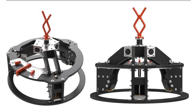
The **AV/AX Ring/Gasket Tool** for removal/installation of AX/VX gaskets is a mechanical tool with no requirement for hydraulic or electric supply from an ROV. This gives the operator the option to transport the tool to/from the worksite without recovery of the ROV. Suitable for use with or without tubing hanger installed in the wellhead.
