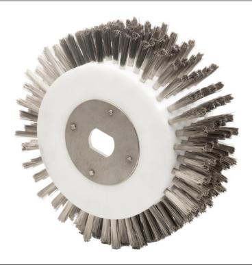
The **Cleaning Brush** is ideal for cleaning soft to very hard marine growth on hard surfaces. To be used with Multi – Purpose ROV Tool 6303-001. Soft or painted surfaces may take damage from this brush.
