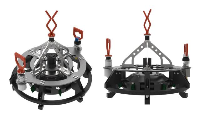
The **Subsea AV/AX Cleaning Tool** is a rotating cleaning tool for the wellhead 18 <sup>3</sup>/<sub>4</sub>" seal surface. An acid injection system is available with a stab system and acid tank. Hydraulic power can be supplied trough hot-stab system or standard hose connections.
