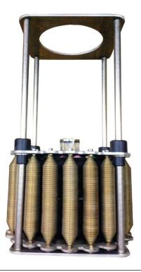
The **45 litre Subsea Compensator** is a general-purpose compensator for underwater hydraulic systems. It provides a given volume and pressure for oil-filled subsea equipment. The compensator consists of a large bellow that is compressed using stainless steel springs. The recommended direction for installation is vertical.
