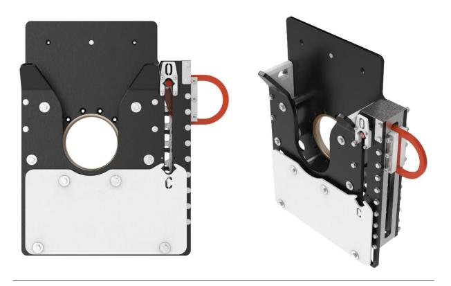
The 6" **Subsea Suction Female Hose Connector** is a low weight ROV operated connector intended for temporary installations subsea. The current system is made to fit 6" hoses and it has 8" full bore through the connector. The connection system does not have any negative impact on the flow. It can be modified to fit hoses in the 2 to 8" size range.
