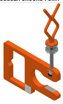
The **Subsea Ground Point** is a universal ground point that can be mounted on metal surfaces. The ground point opening is placed onto the structure and secured in place by operating the ROV handle. The structure is designed tension up when the handle is turned and tightened up. This in combination with two-disc springs in the ROV handle mechanism ensures that the ground point is properly secured to the metal.
