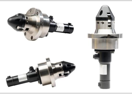
The **Docking Probe** is Ideal for docking of ROV, ROV/RIT tools. The docking probe is hydraulically operated and has a failsafe mechanism that will automatically release in a power failure situation.
